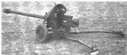
The PAK 57 is identified from the PAK 50 by its curved gun shield.
