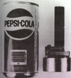
A machinist built this gun-in-a Pepsi-can for Mr. Fink's collection. It's a well-disguised .50-caliber percussion pistol built into the can. (Courtesy of David H. Fink)
