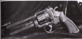
Pat Scrufari's over/under modification as tested by the U.S. Army as a survival pistol. The top of this heavily altered Smith & Wesson is .22, the lower a .357. (Courtesy of Pat Scrufari.)
