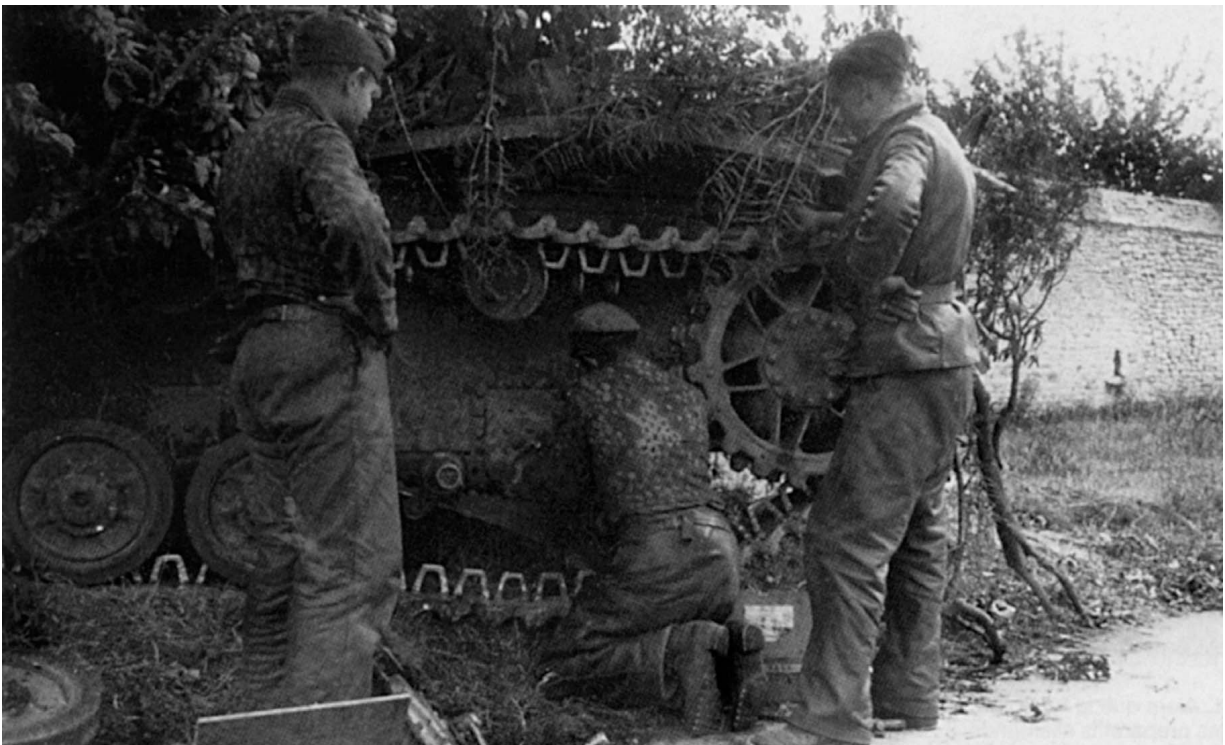
The crew of a Panzer IV carry out repairs on the running gear of their tank.
