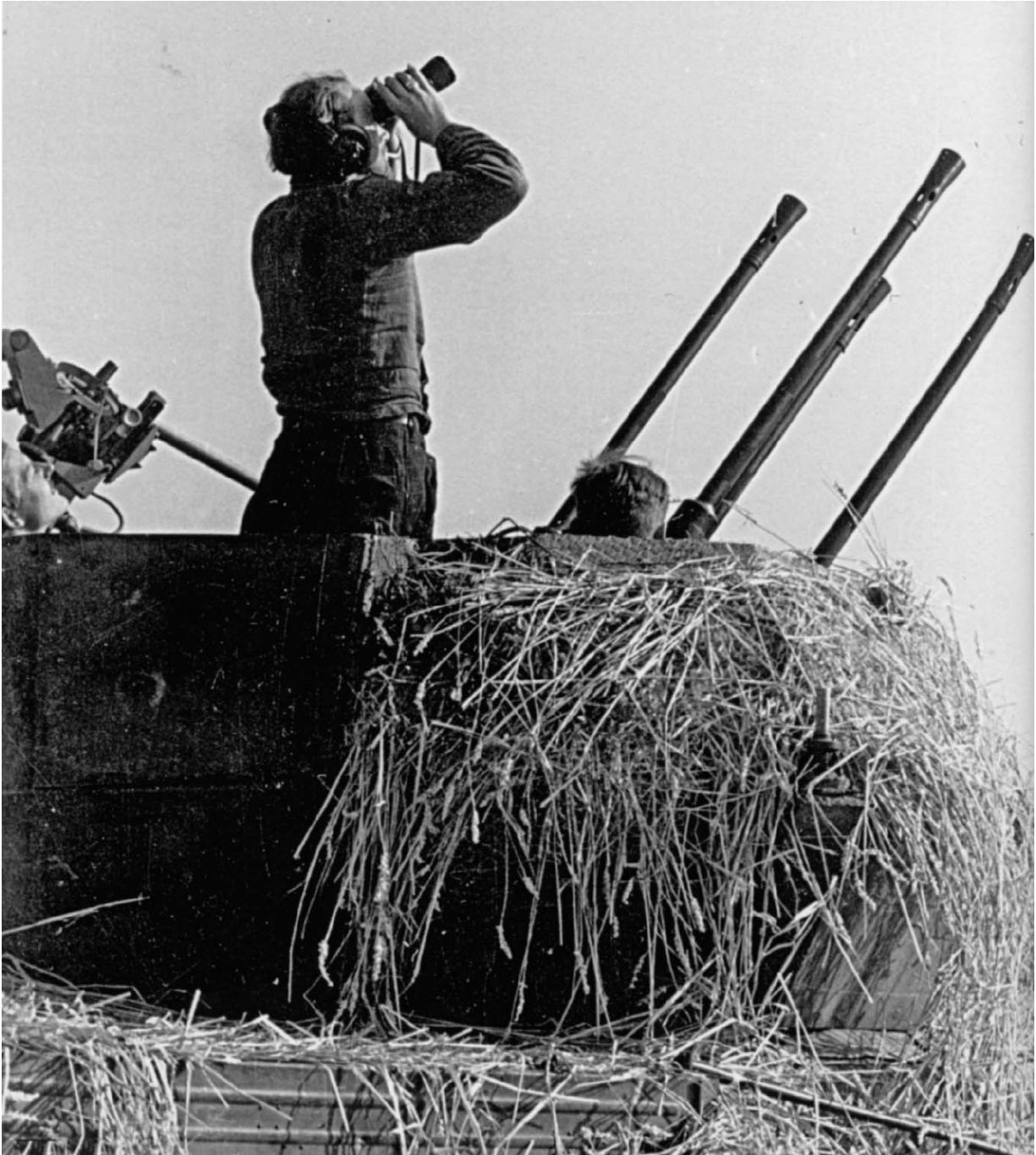
The 20mm Flakvierling on the hull of a Mark IV Panzer.
