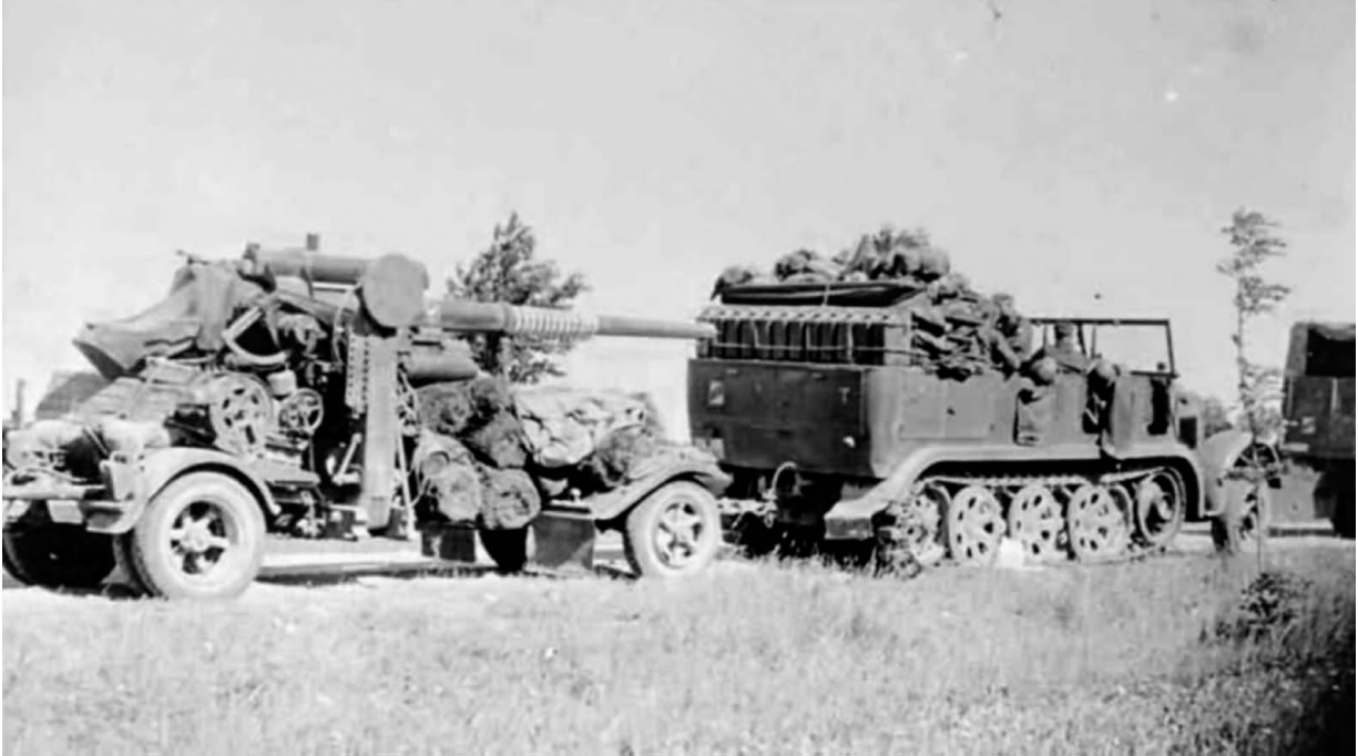
The 88mm Flak 36/37 and its prime mover the Sd.Kfz.7, as issued to III Flak Corps.
