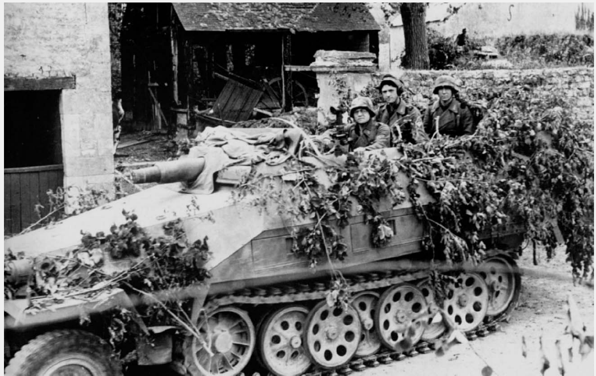
An early version of 'Hanomag' mounting the 75mm 'Stummel' as issued to the Hitlerjugend .
