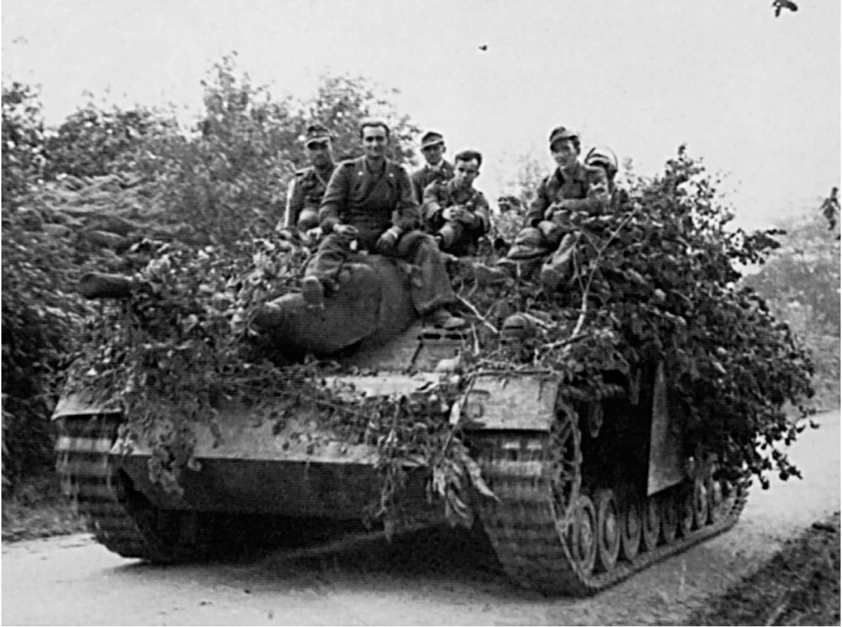
A Jagdpanzer IV, mounting the same L48 75mm gun as the Panzer IV.
