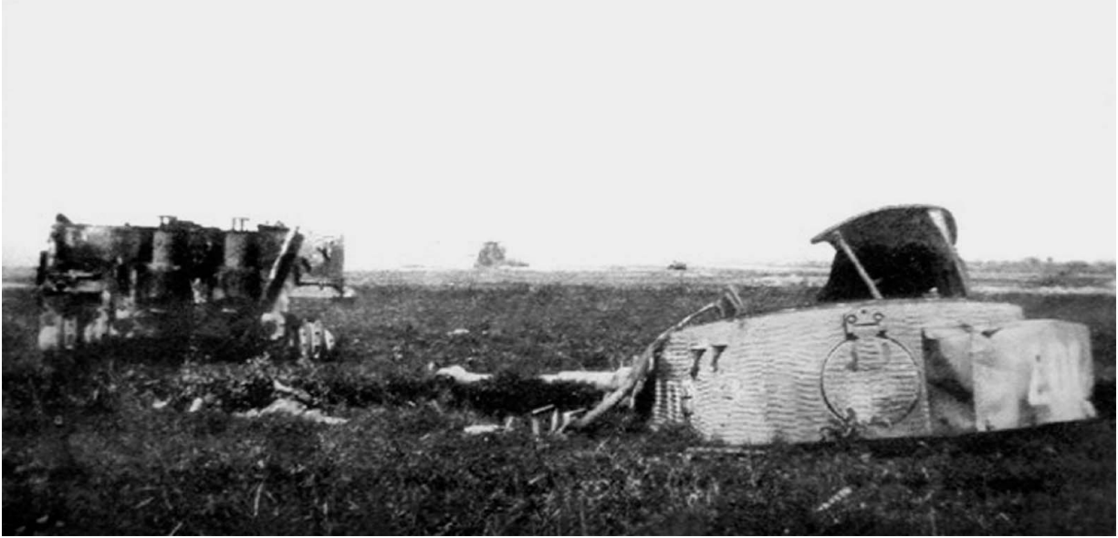
Wittmann's Tiger 007 with its turret displaced by the internal explosion and by being moved to remove the tracks.
