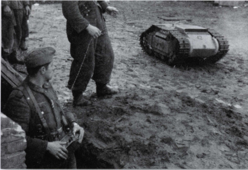
German pioneers preparing a Goliath demolition vehicle for an attack on a Polish barricade. The Goliath could carry a 75kg charge that was powerful enough to demolish reinforced concrete structures, but its control wires were vulnerable to damage and the vehicle was rather slow, with a top speed of only 10km/h. (Bundesarchiv, 101III-Ahrens-026-12)
