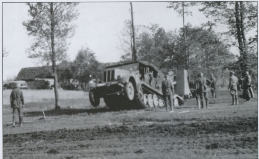
Sd.Kfz.7 half-track prime mover seems to be having trouble negotiating uneven ground while towing an "88."
