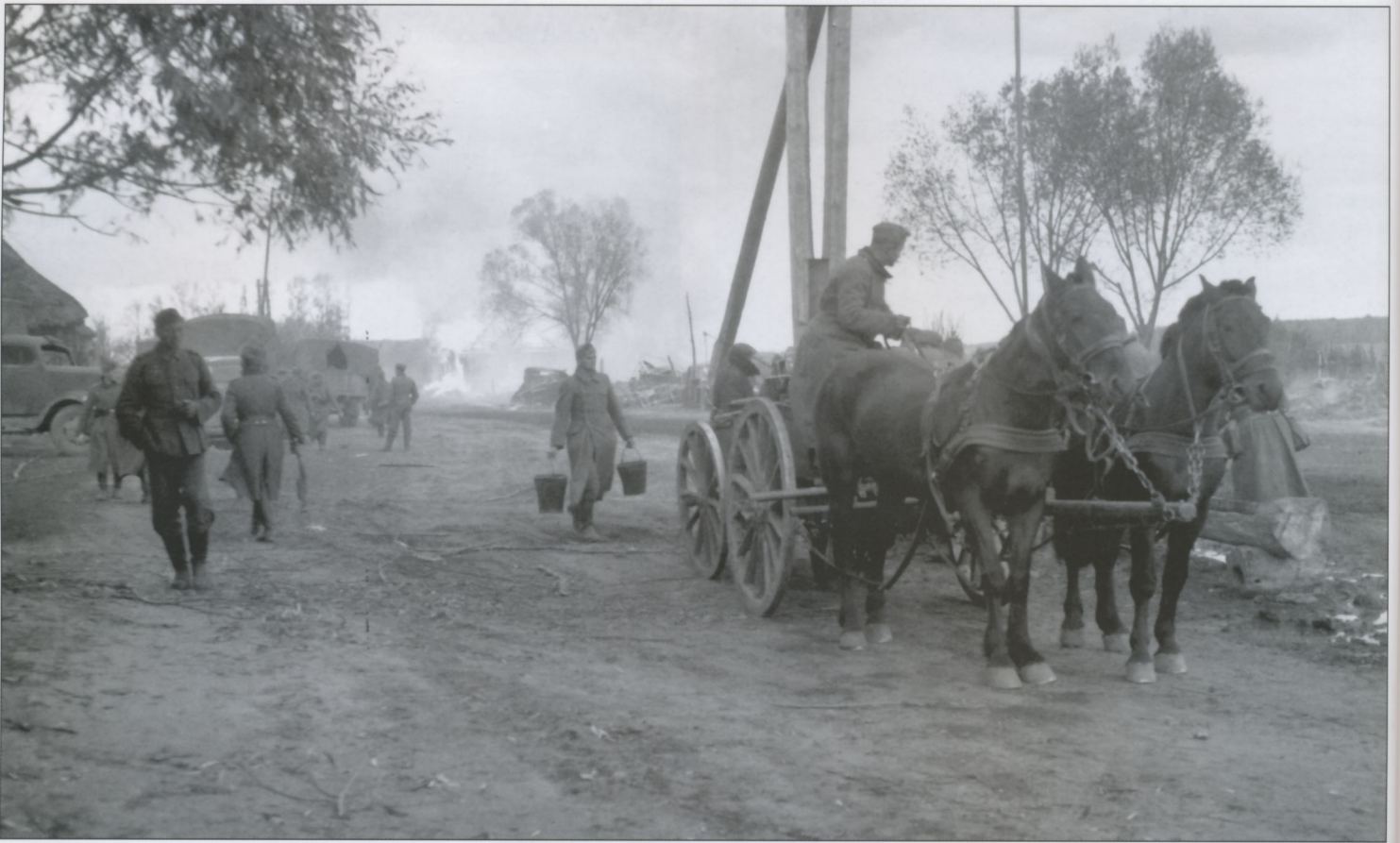
Two photos of a Gulashkanone field kitchen. The Fissler Company made the initial design in 1892. These newer versions had a 200l stewpot and 90l coffee pot, enough to serve approximately 120 troops. In lower photo Soviet POWs are preparing food as "volunteers."
