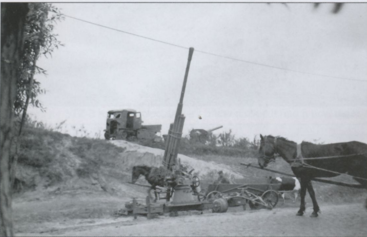
Civilians with their horses and cow mill around destroyed Soviet ordnance. Pointed skyward is an 85mm M1939 anti-aircraft gun. Behind it is a 122mm M1938 howitzer and its prime mover.
