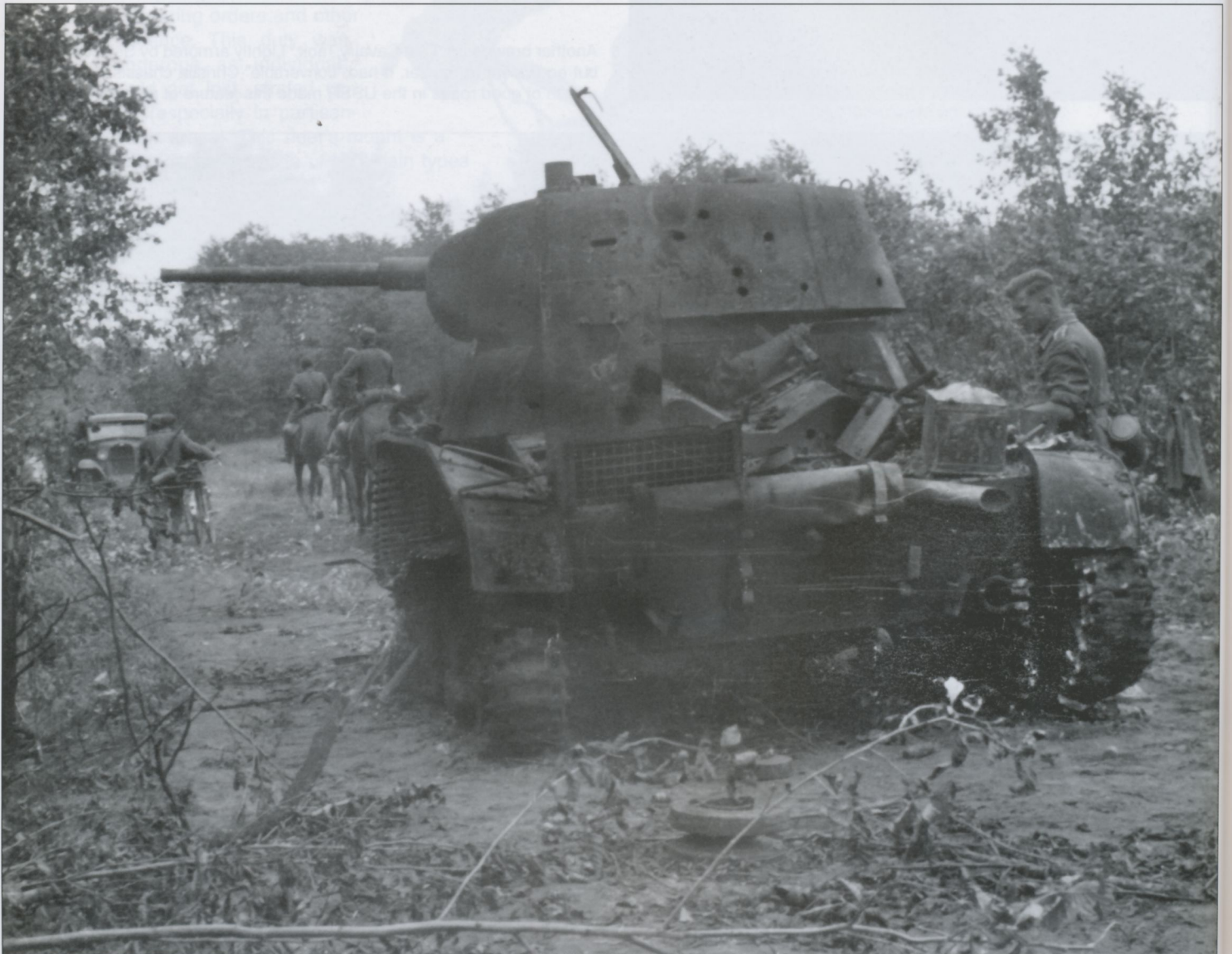
A destroyed T-26S. This was an improved version of the T-26, introduced in 1939. It had a new turret and welded, sloped hull sides.
