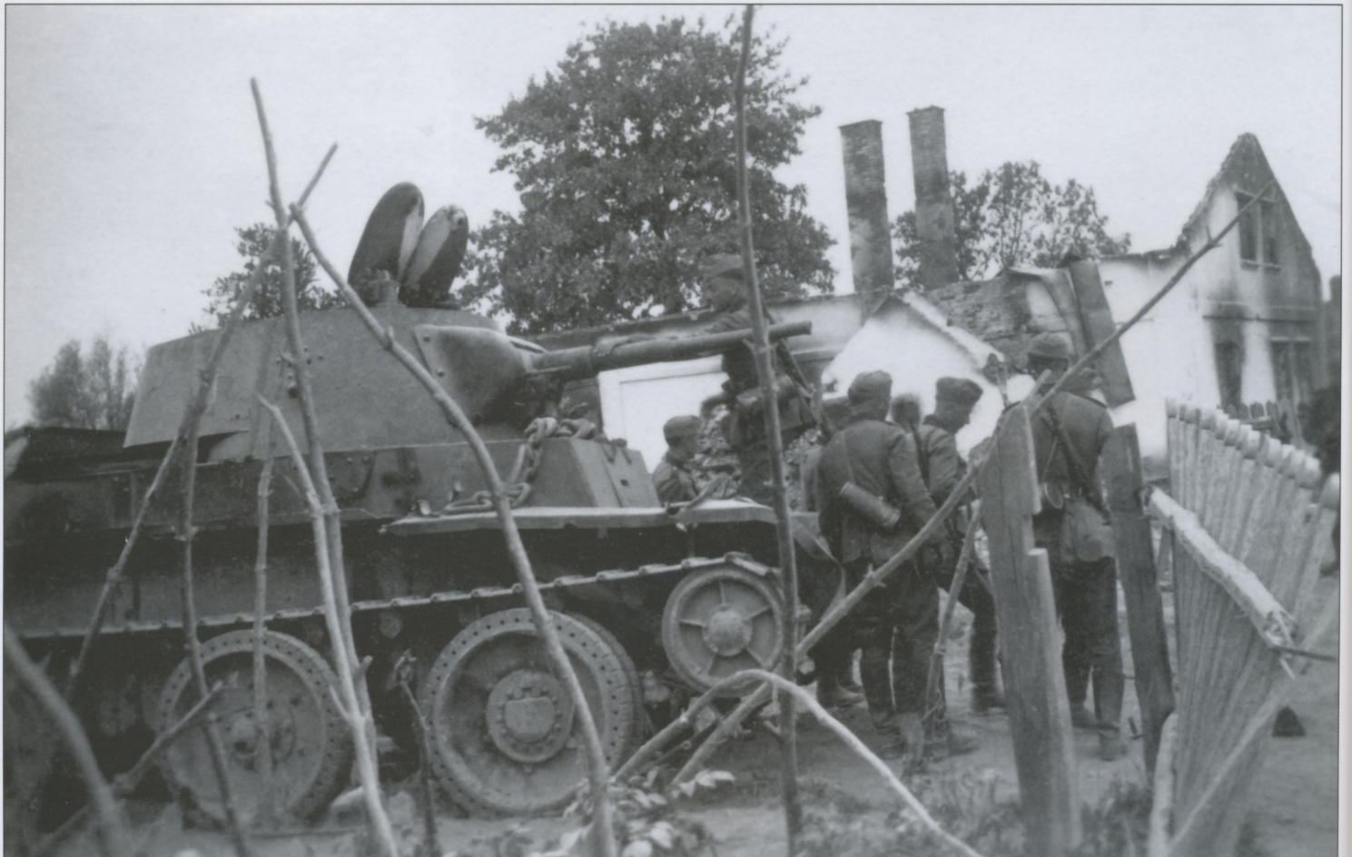
Abandoned 14-ton BT-7 "Fast Cavalry Tank." A fully loaded BT-7 carried 145 main-gun rounds. Most tanks of this type had disappeared by 1942.
