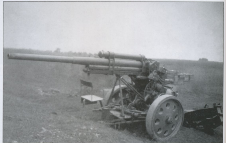
A 76mm M1938 anti-aircraft gun, precursor of the M1939. Note lack of muzzle break.
