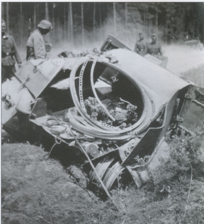
These Germans are very curious about a disabled BA-6 5-ton armored car. The chassis was based on a 4x6 Ford truck, it mounted the same 45mm gun as the T-26 plus two machine guns.
