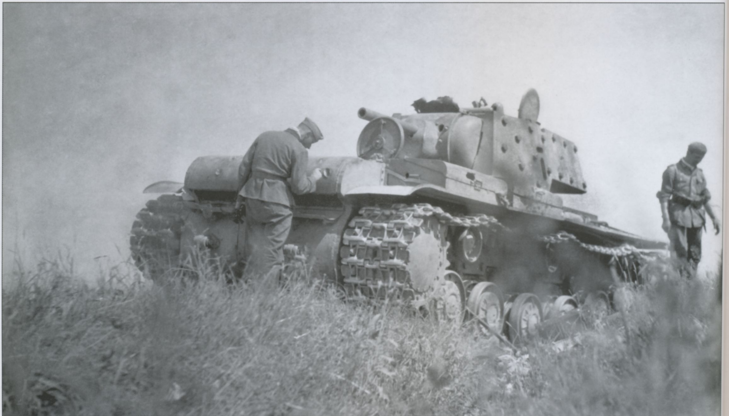
A massive 45-ton KV-1. It mounted a 76mm main gun and four machine guns and was protected by up to 90mm of armor. It won the competition for a new Red Army heavy tank after other types did poorly in the Winter War against Finland in 1939-40.
