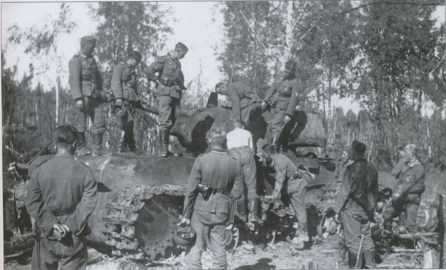
Germans climb over a destroyed KV-1 while an NCO looks on (right). The KV-1 was underpowered, had an unreliable transmission and was hard to steer, but the Germans required all the ingenuity they could muster to halt one.
