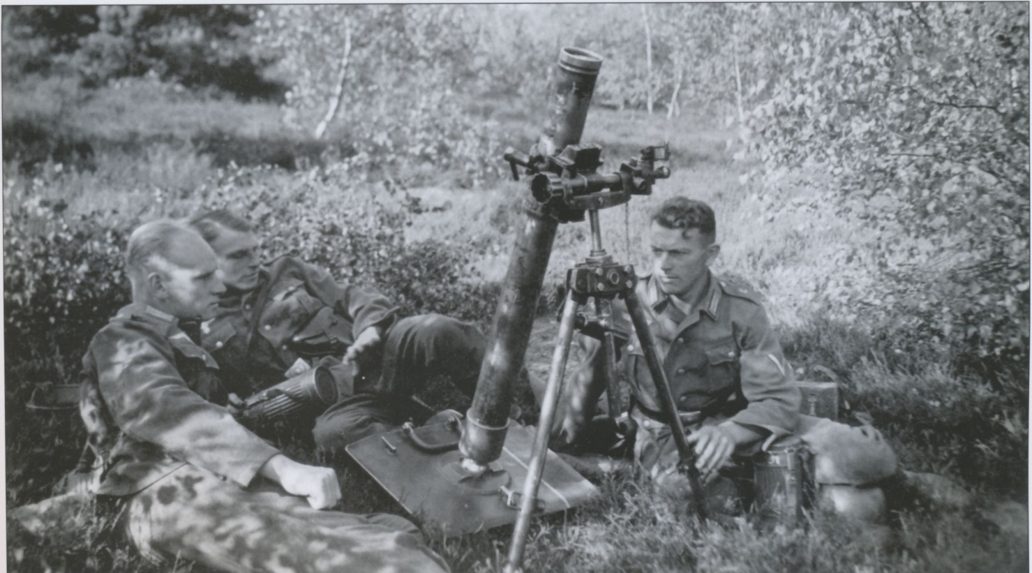
An 8cm Grenatenwerfer 34 Mortar and crew, led by Gefreiter on right. Rheinmetall developed this battalion weapon in 1932 and it was deployed in 1937. It weighed 57kg and consisted of tube, bipod and base plate. It had a range of 2400m.
