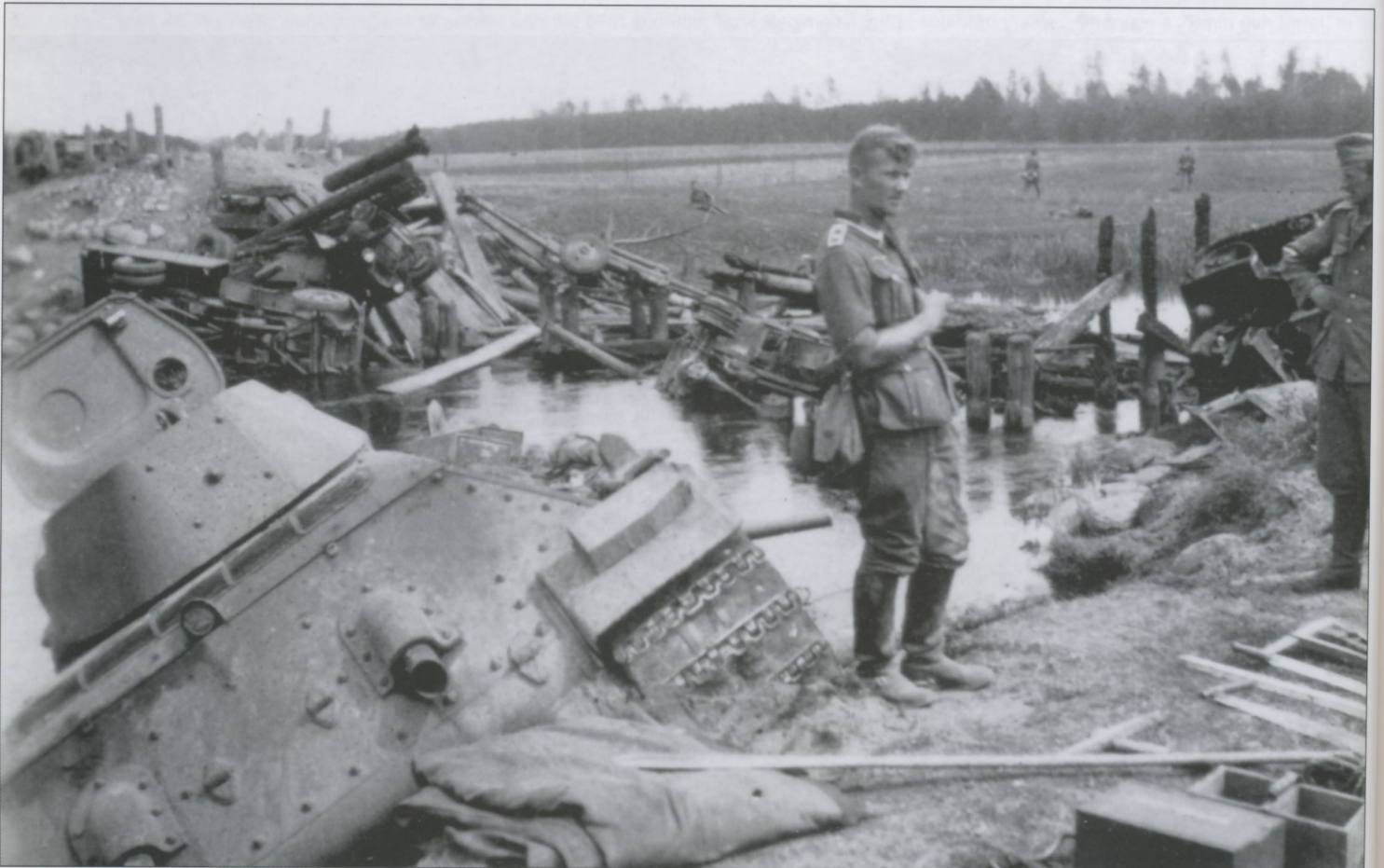
A T-34, the Second World War's best tank until the arrival of the Panther, in this case squandered when it was driven onto bridge too weak for its weight. In the center is a senior NCO.
