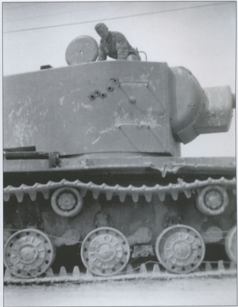
A Gefreiter atop the turret of a massive KV-2 infantry support tank. Its official name was "Heavy Artillery Tank," but its crews nicknamed it "the Dreadnought." This particular vehicle took at least five hits to the turret, none of which penetrated its armor.
