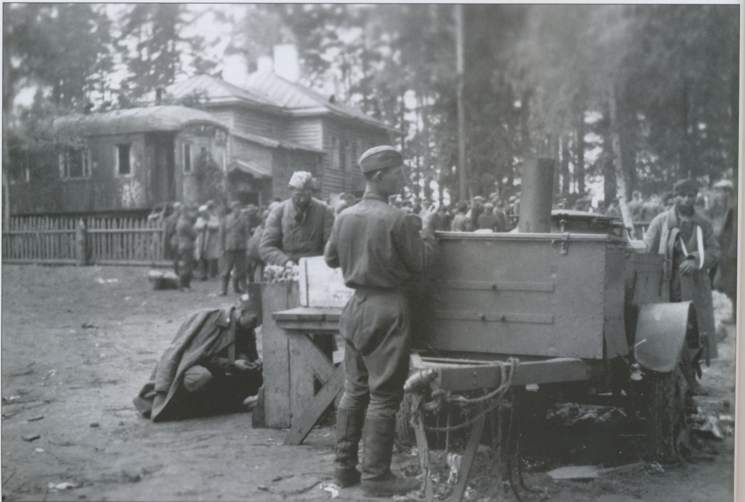
Two photos of a Gulashkanone field kitchen. The Fissler Company made the initial design in 1892. These newer versions had a 200l stewpot and 90l coffee pot, enough to serve approximately 120 troops. In lower photo Soviet POWs are preparing food as "volunteers."
