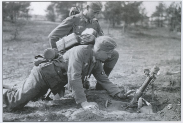
The 5cm Grenatenwerfer 36 mortar gave the infantry company its own fire support. The Rheinmetall weapon weighed 12.5kg and came in two pieces: tube and base plate. Man in foreground wears grenadier's qualification patch on his left sleeve and a box of ammo on his back.
