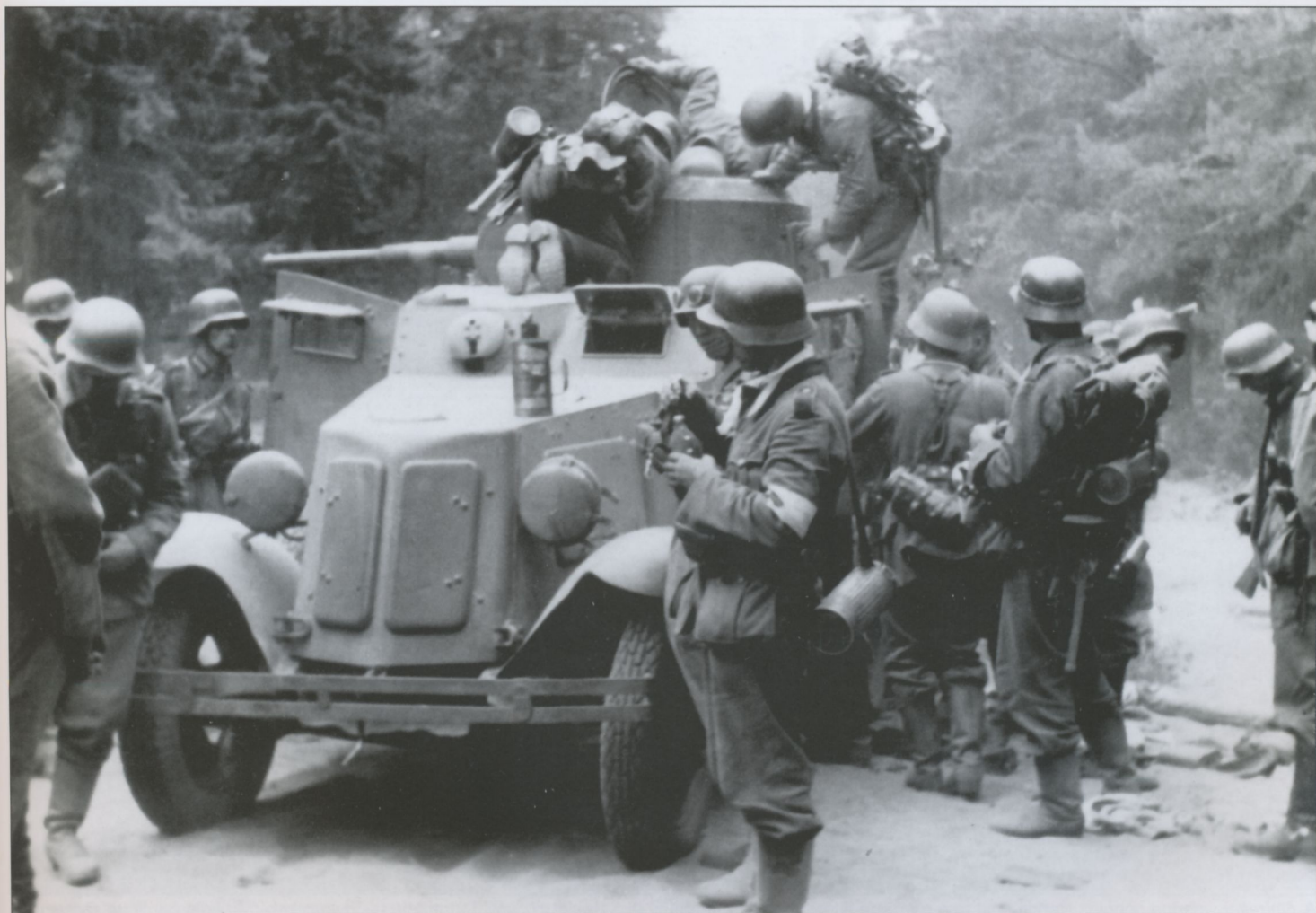
These Germans are very curious about a disabled BA-6 5-ton armored car. The chassis was based on a 4x6 Ford truck, it mounted the same 45mm gun as the T-26 plus two machine guns.
