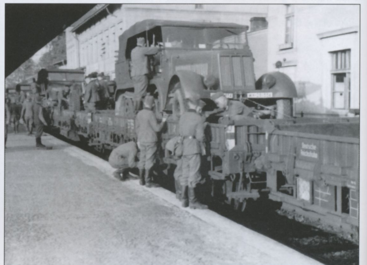
Soldiers prepare vehicles for a rail trip, the most efficient way to move large units long distances. The men are securing Sd.Kfz.7s to the rail cars. These cars are clearly marked "Deutsche Reichsbahn," meaning the Germans have converted the Soviet rail gauge to their use.
