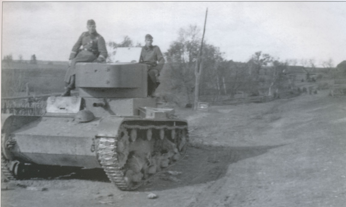
Two Germans inspect a T-26. Compare the vertical slab sides of the turret and hull to the T-26S. This tank model saw success during the Spanish Civil War and at Khalkin Gol, but was reaching obsolescence in 1941.
