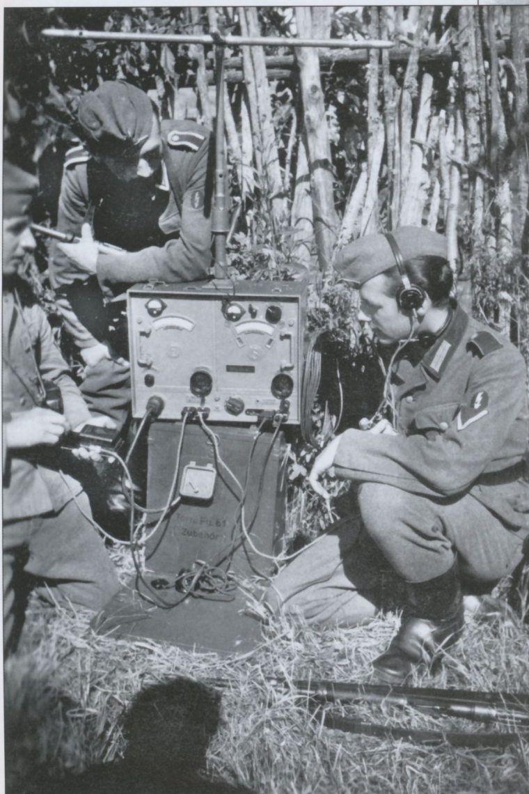
An NCO leans over Torn.Fu.b1 while a Gefreiter operates the radio, both men wear signal troops qualification badges on their sleeves. The Torn.Fu.b1 was made up of three parts: Receiver (top left) and receiver (top right) and power supply (bottom).
