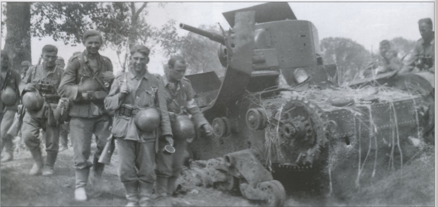
German soldiers, including a medic (center) pass a brewed-up T-26 light tank. Based on the British 6-ton Vickers tank, this successful 1930s design made up the bulk of the Soviet tank force during Barbarossa. Over 12,000 were produced, mounting a 45mm gun.
