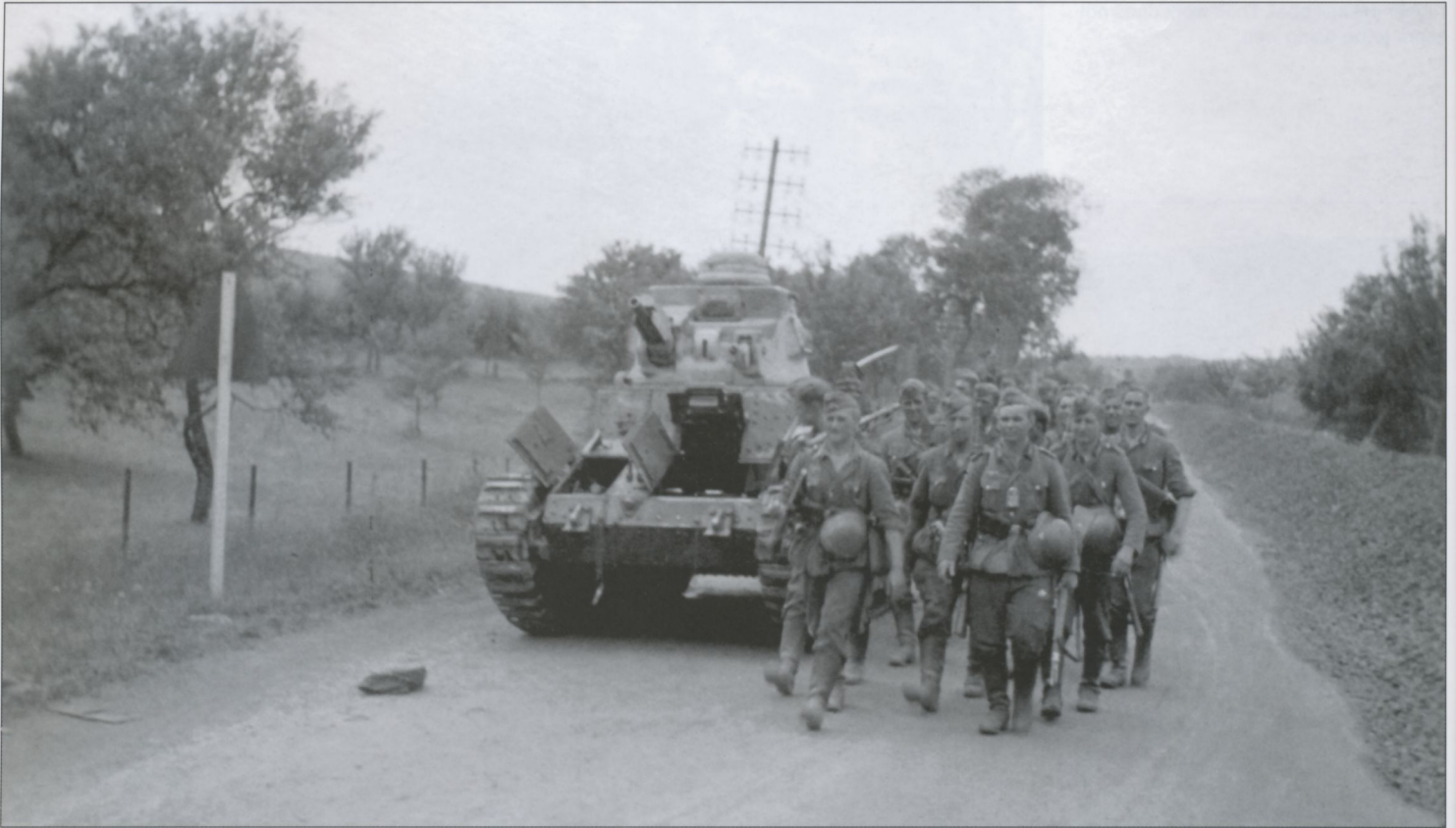
German soldiers march around a destroyed T-18 light tank. Symbolic of Soviet weakness during the early days of Barbarossa, this unsuccessful design was among the Red Army's first. Based on the French Renault, the 6-ton tank mounted a 37mm gun.
