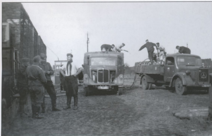
Undoubtedly at a rear-area base, Daimler-Benz L3000 loaded with barrels transfers fuel to another truck. The Wehrmacht did not have many specialized fuel tanker trucks including powered pumps, so most fuel transfers were done using the slow and labor-intensive hand pump method and small barrels or even smaller "jerry cans."
