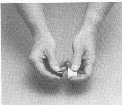
Epoxy thread protector into 3/4" x 1/2" bushing.
