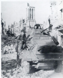
Below: An SdKfz 231 eight-wheeled armoured car from the Hitler Jugend Division amidst the ruins of a French town. The 12th SS-Panzer Division Hitler Jugend was an attached unit to 1 SS-Panzer Corps during the Battle of Normandy.
