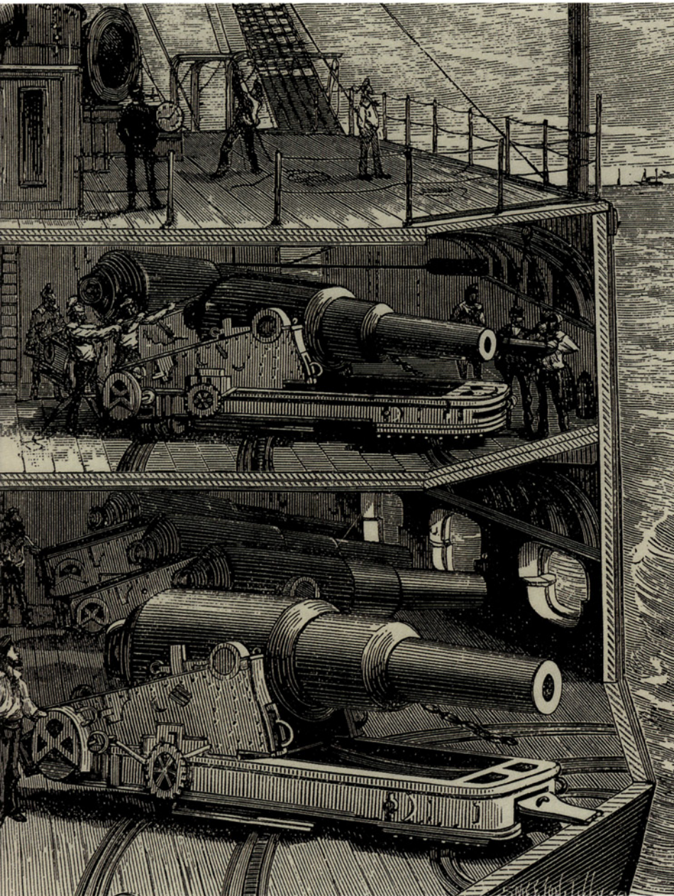
HMS Alexandra was not just a pretty flagship: this picture of her centre battery shows the disposition of the heavy guns to enable them to fire over relatively wide angles of bearing.
