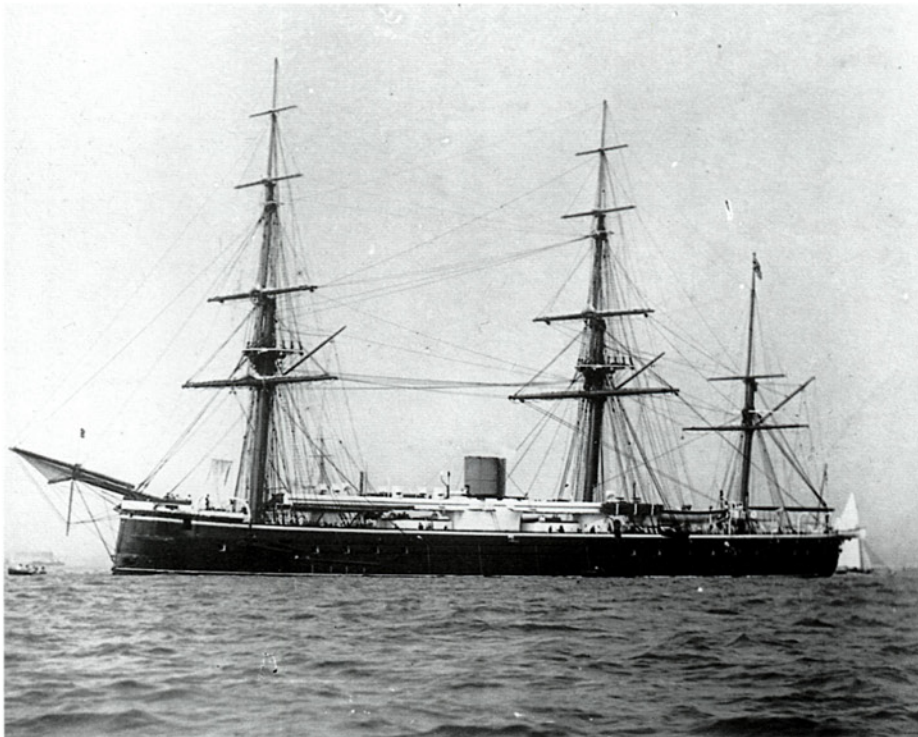
HMS Monarch, 1871. A high-freeboard turret-ship, much safer than the ill-fated Captain, she nevertheless suffered from the belt-and-braces approach that gave her a full sailing rig as well as steam power. Note the massive construction of the masts, an impediment to fighting ability.
