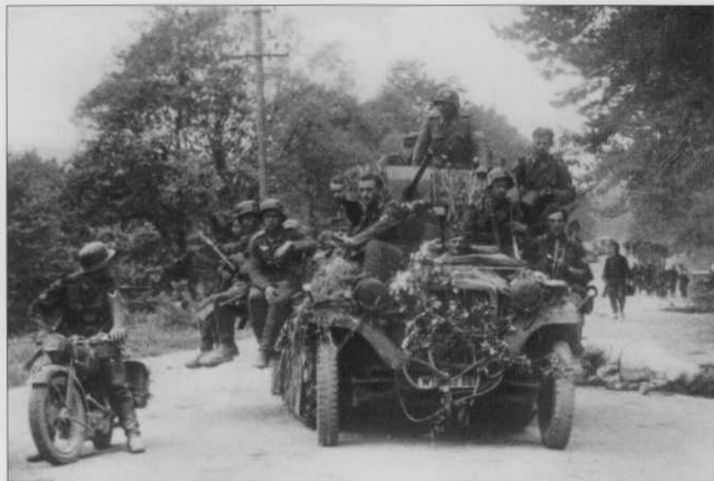
An SdKfz 10/4 halftrack operating on the Minsk-Moscow highway in autumn 1941. Each motorized Panzerjäger battalion had a platoon of four SdKfz 10/4 halftracks with a single 20mm gun. (Nik Cornish)
