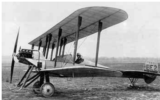
BE2c built by British & Colonial ("Bristol"), and powered by the 90 hp RAF 1A engine
